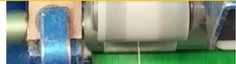
**Microspinning, Cirad-LTC, ring-spinning, 20 tex yarn, 23°C & 55%RH**
