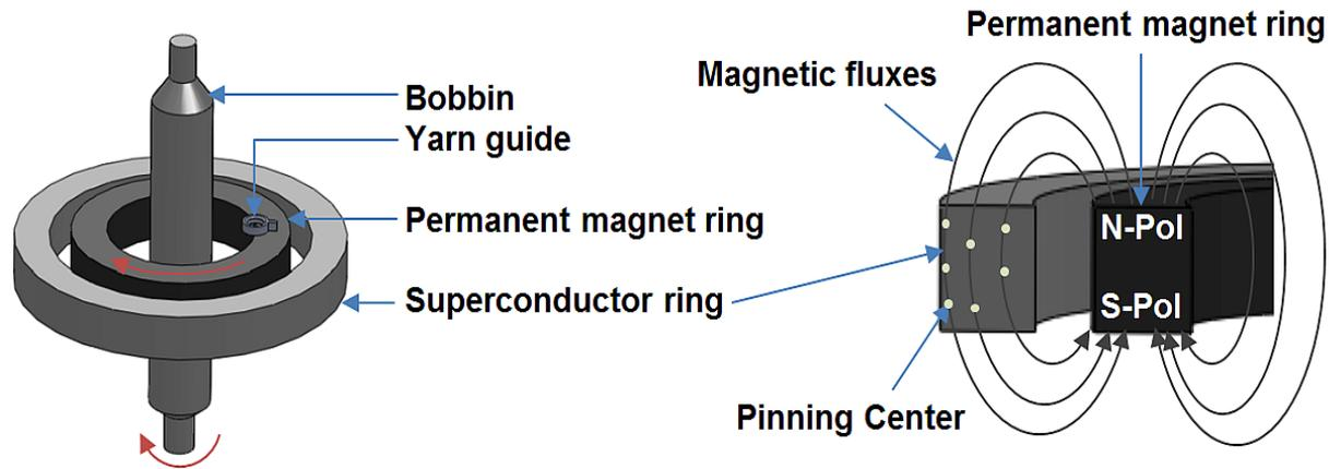
Concept 2: Topology and cross-sectional view, where magnetic fluxes are trapped in pinning center
