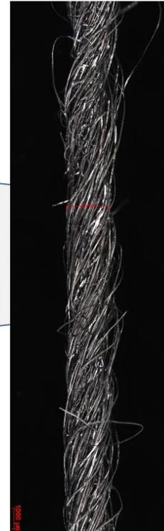
Fabric structure made of 100% metal spun yarn
