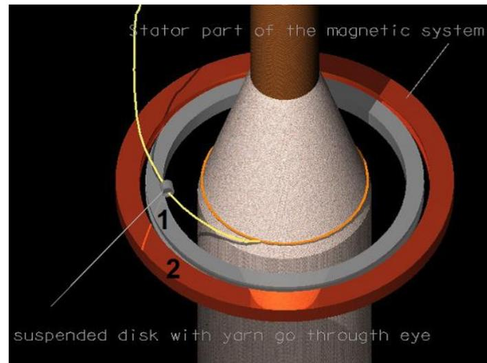
Electrically controlled ring with a levitated ring|© US Patent 7205692
