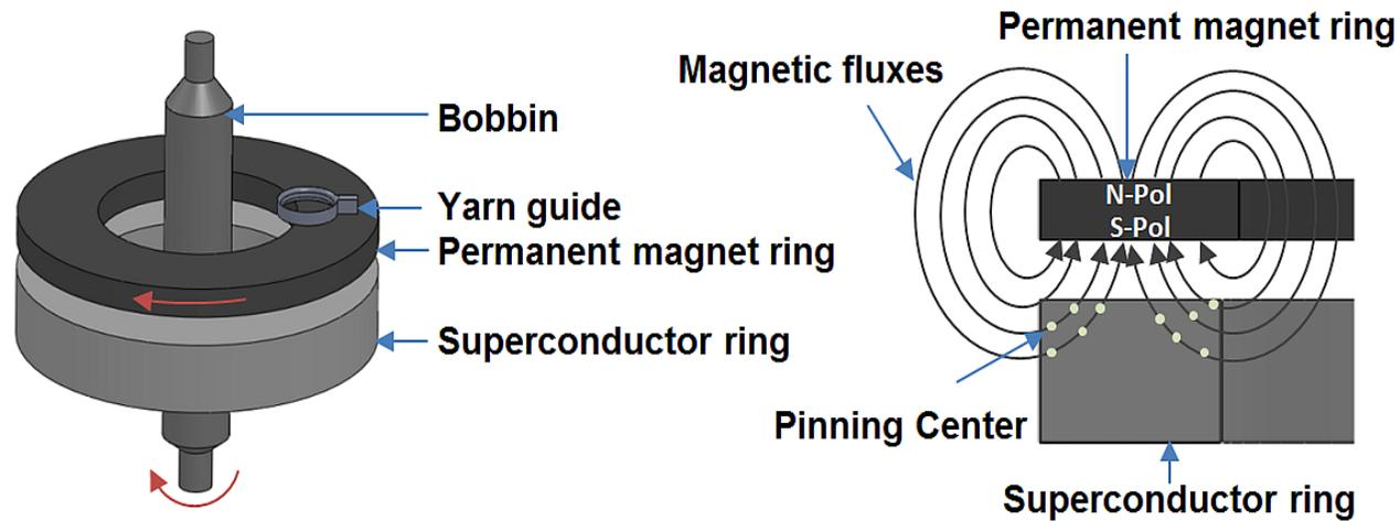
Concept 1: Topology and cross-sectional view, where magnetic fluxes are trapped in pinning center
