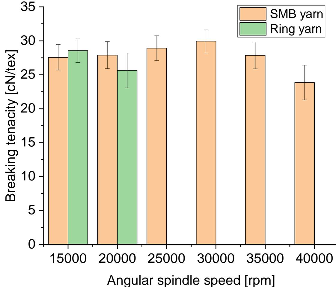
Comparison of yarn strength of conventional and SMB ring yarn from 100% cotton material for different angular spindle speeds (yarn count 20 tex)
