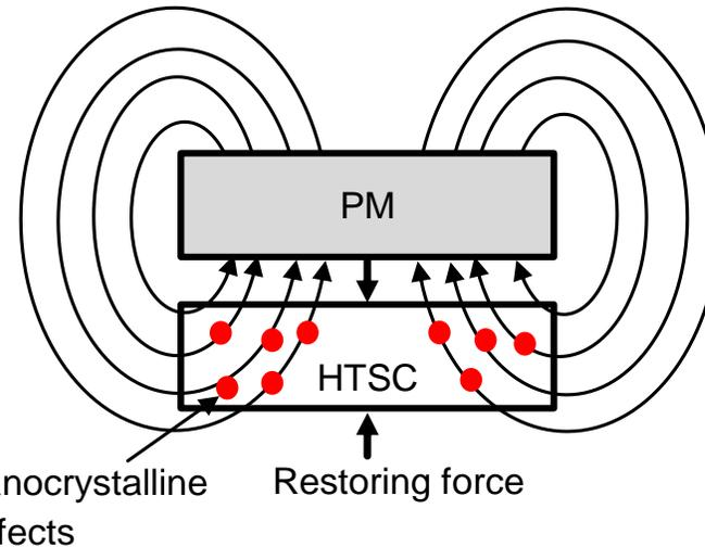
Functional principle of superconducting magnetic bearing (SMB)
