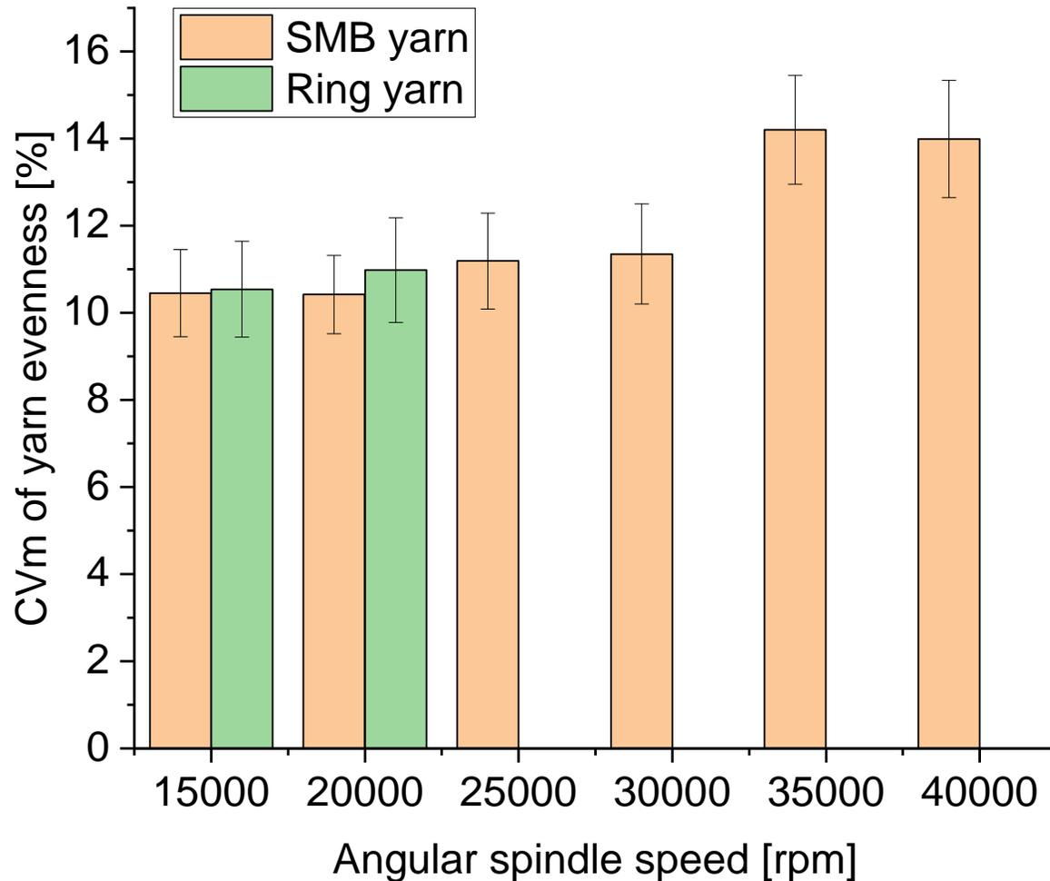
Comparison of yarn evenness of conventional and SMB ring yarn from 100% cotton material for different angular spindle speeds (yarn count 20 tex)
