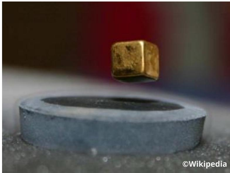
A magnet levitates above a high temperature superconductor cooled with liquid nitrogen (-196°C)
