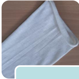
Knitted tube (raw fabric)
